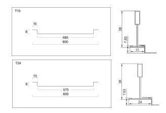
Fire reaction pre and postpainted tiles: A2s1do Release of dangerous sustances: none Flexion resistance: Classe 1 Durability galvanized tiles: B Durability pre and post-painted tiles: C
